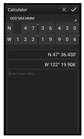
c:geo offers a calculator for waypoints, which allows to make use of variables and formulas to calculate coordinates based on the result.
